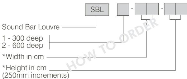
\*When ordering, allow for 10mm all around the louvre to accommodate for site discrepancies.
